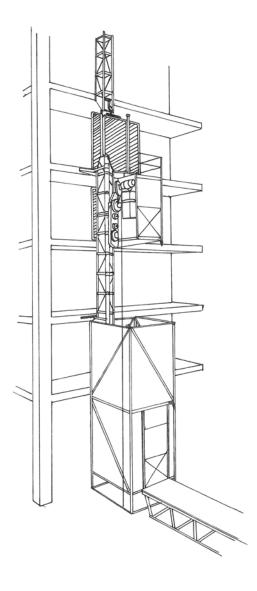
A materials or personnel hoist is a cantilevered hoist, a tower hoist or several winches configured to operate as a hoist and is intended to carry goods, materials or people.
