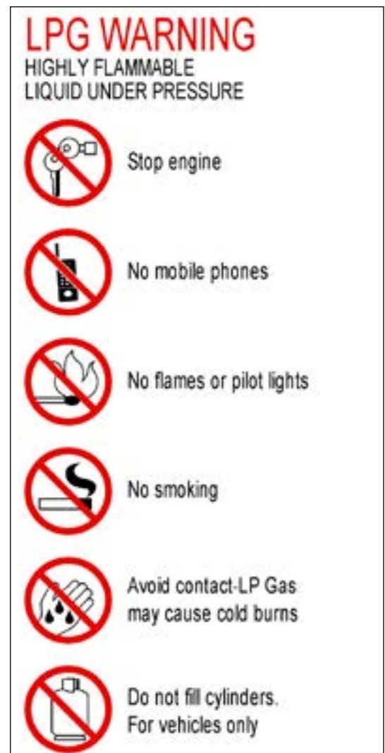
Example of LP Gas filling warning sign (not actual size)
