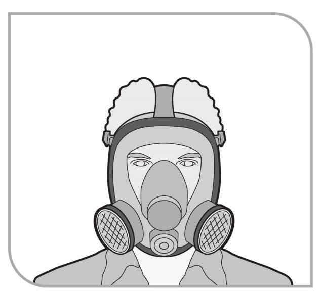
Figure 12 Full-face, particulate filter (cartridge) respirator
