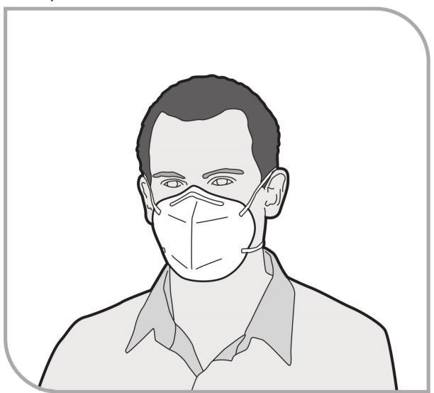
Figure 9 Disposable, half-face particulate respirator
