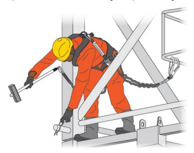
Figure 7 Fall arrest system used during tower crane assembly
