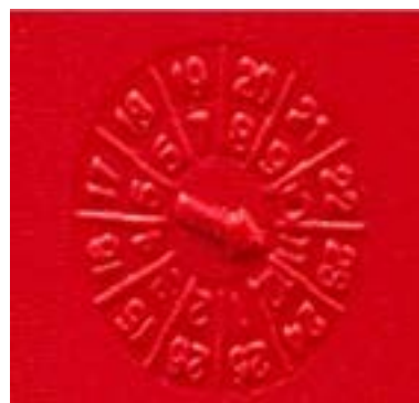
Figure 2: Example date of manufacture code. Inner circle = month; outer circle = year. This container was manufactured in November 2023.
