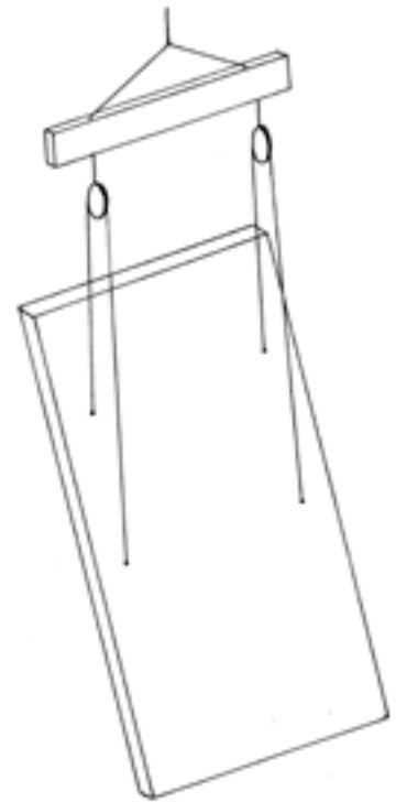
Tilt Slab with loading equaliser gear
