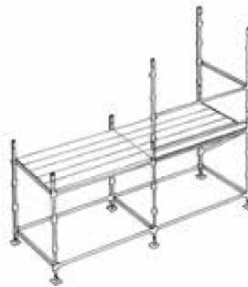
Prefabricated scaffold (modular type)
