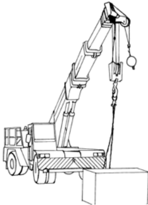
Non-slewing mobile crane (includes lattice and hydraulic boom types)
