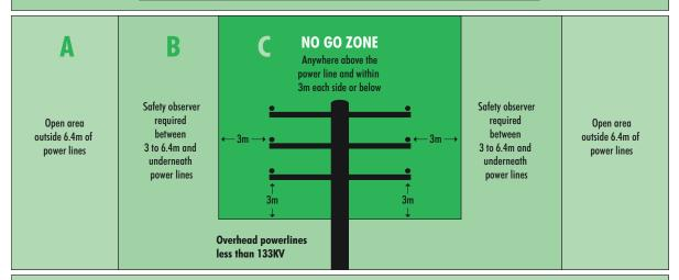
A SAFETY OBSERVER is required when working under Power Lines
