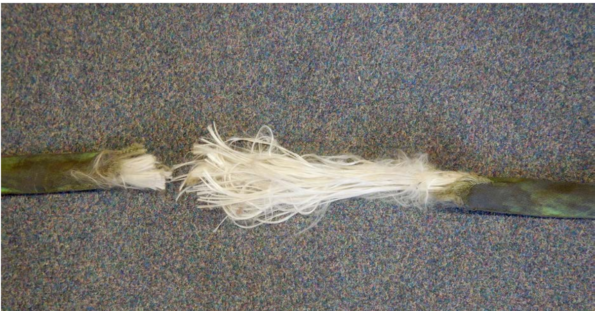
Failed sling showing damage from sharp edge
